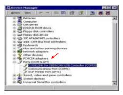
Click 'Port (COM & LPT)' you will see 'CODELINK for OBD&CAN USB Controller (COM3)' the CreaderV has been connected at COM3.
